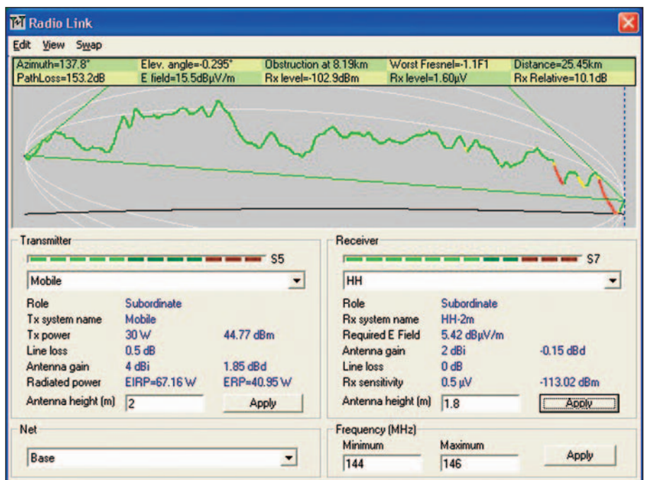
FIGURE 3: POOR LINK QUALITY ALONG THE PATH IS SHOWN IN YELLOW, UNUSABLE QUALITY IS RED
